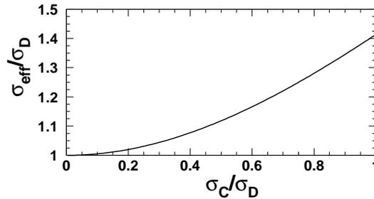
Fig. 8.1: Effective detector precision as a function of calibration precision.
