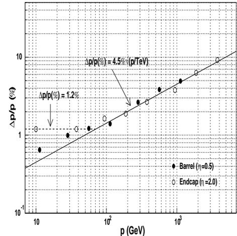
**Fig. 1.2:** Combined CMS Tracker and Muon Chamber momentum resolution as a function of momentum, in the central and forward rapidity regions.
