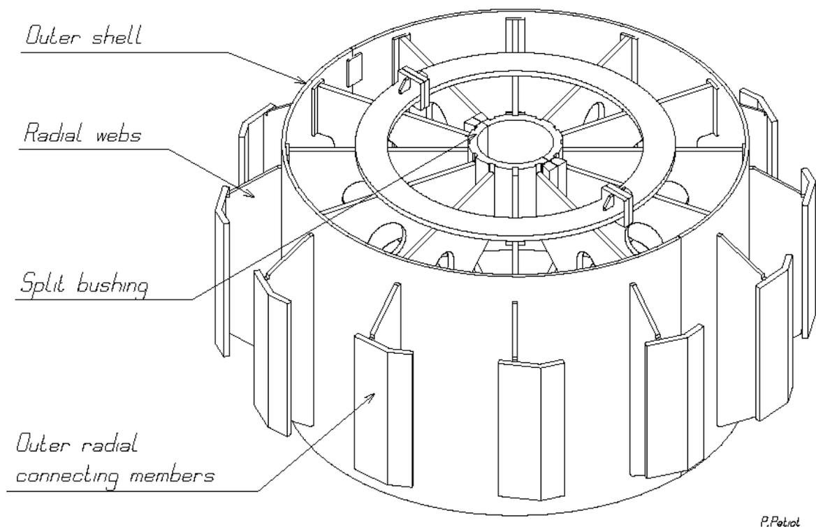
**Fig. 9.4:** Central section of the outer shell. This will be used as assembly jig in the Ferris Wheel for the central barrel yoke.
