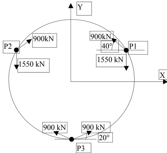
**Fig. 9.2:** Reactions of the cold mass supporting system.
