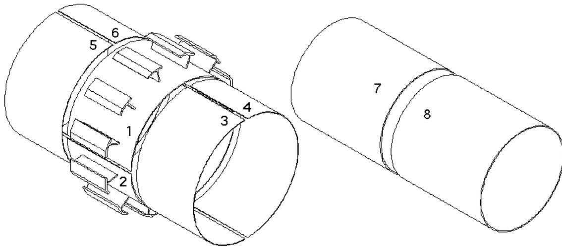
**Fig. 9.3:** Split outer and inner shell.
