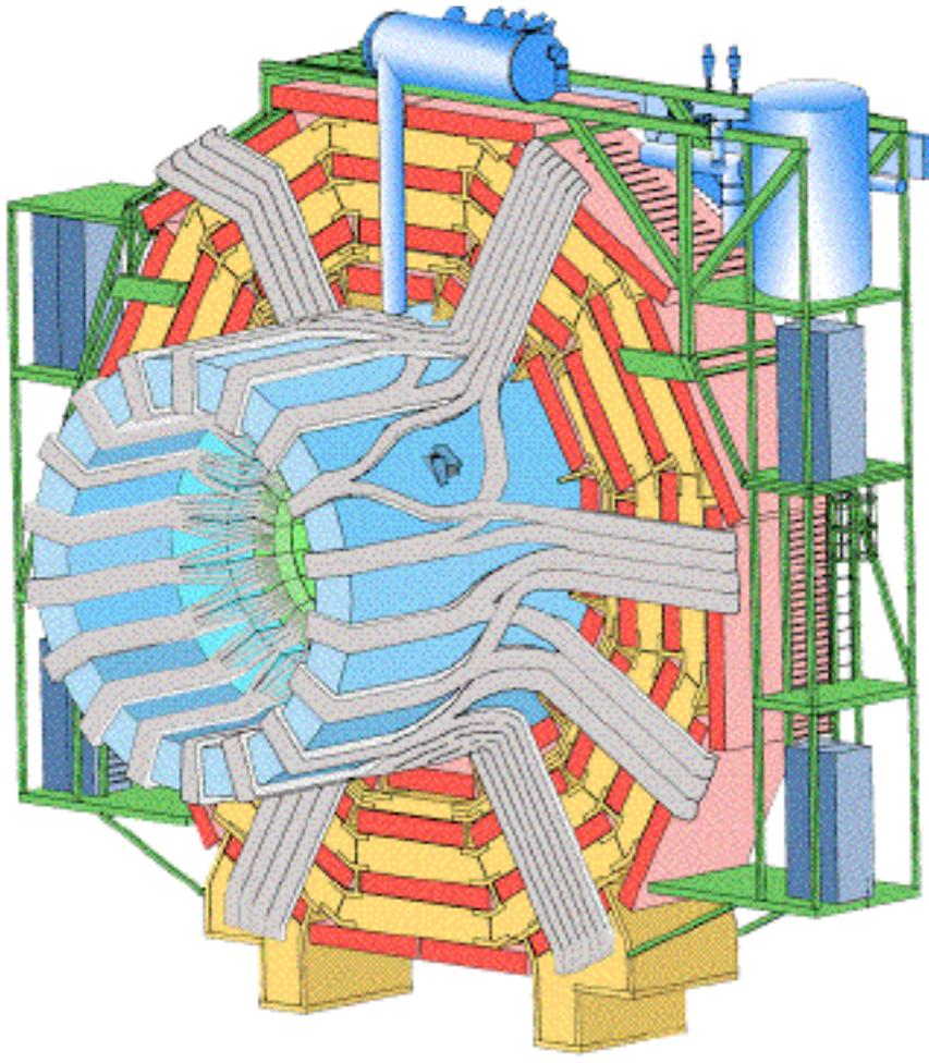
**Fig. 4.1:** The routing of cables and services from the inner barrel detectors over the vacuum tank, and along the barrel ring YB0
