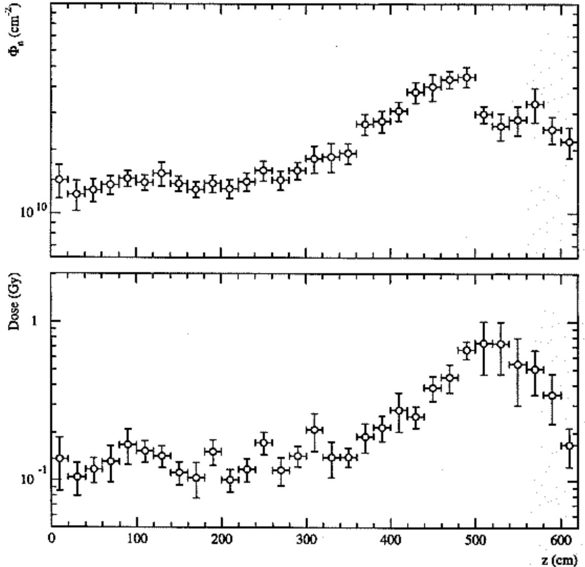
**Fig. 29.2:** Neutron fluence and radiation dose in the superconducting coil. Values are for  $5 \times 10^5$  pb<sup>-1</sup>. The error bars indicate only the statistics of the simulations.
