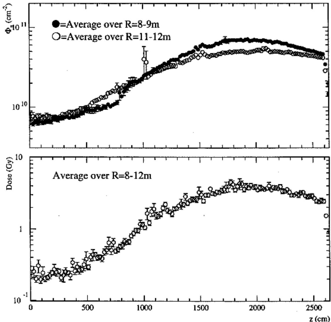
**Fig. 29.1:** Neutron fluence and radiation dose close to the lateral wall of the CMS experimental hall. Values are for  $5 \times 10^5$   $\text{pb}^{-1}$ . The error bars indicate only the statistics of the simulations.
