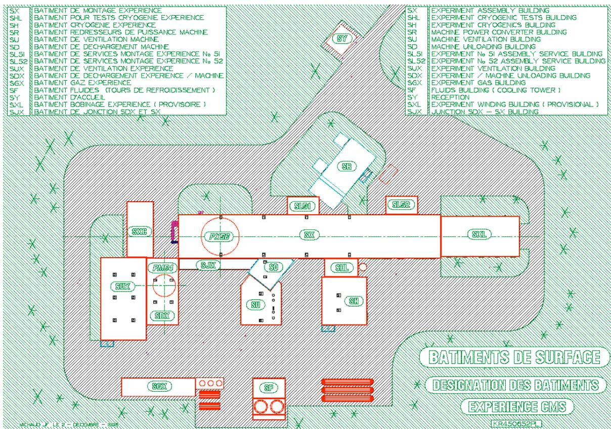
Fig. 25.1: General view of the surface building layout at Point 5
