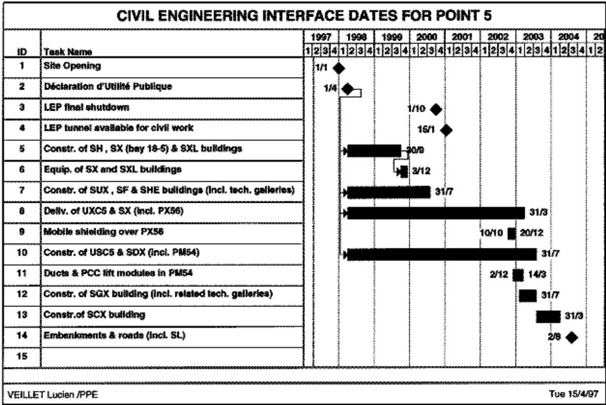
Fig. 25.6: Construction planning for the experimental hall.
