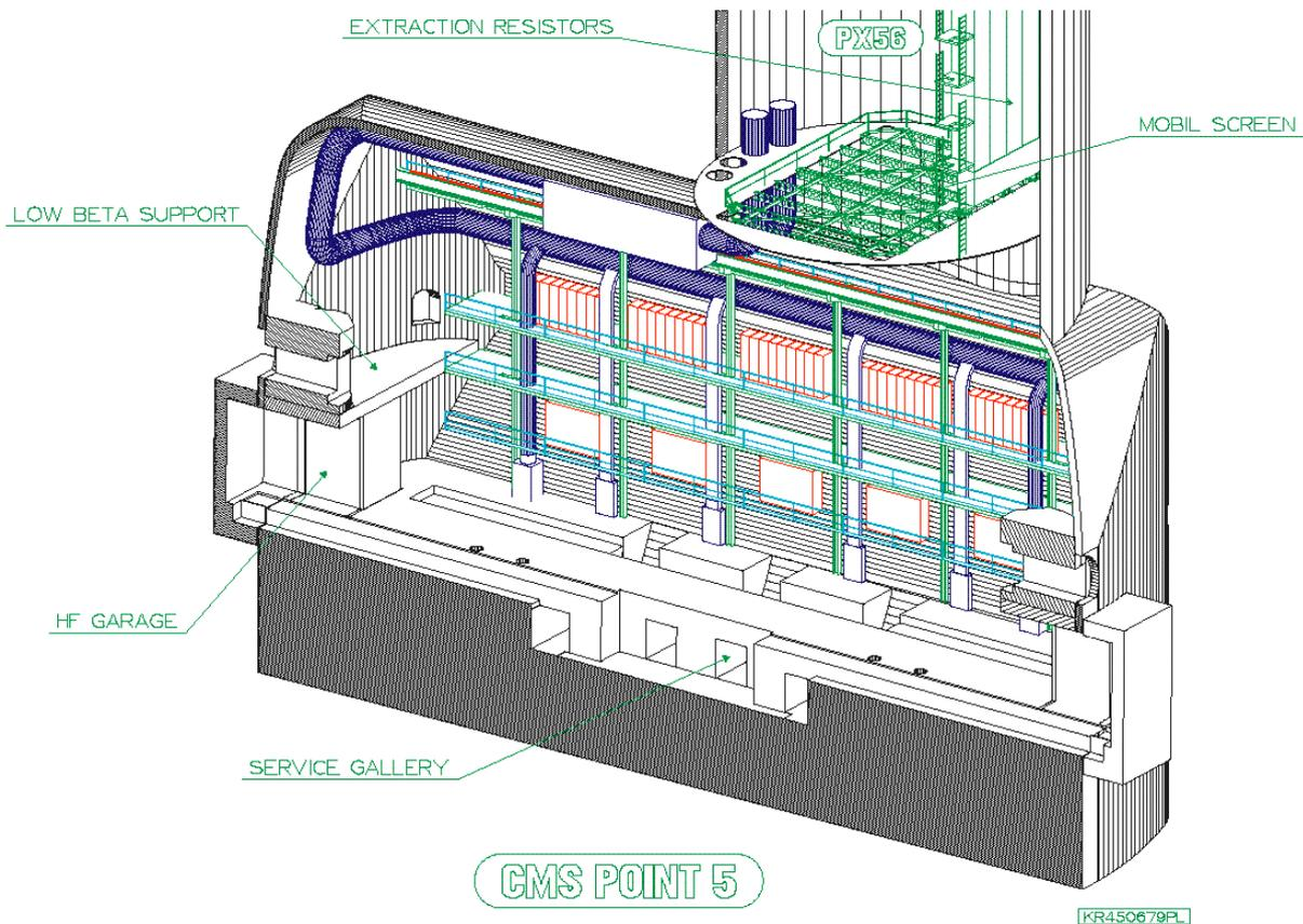
**Fig. 25.4:** Detailed view of experiment cavern showing the protection platform in the access shaft, the low  $\beta$  concrete platform and the 'garage' for the HF detectors.
