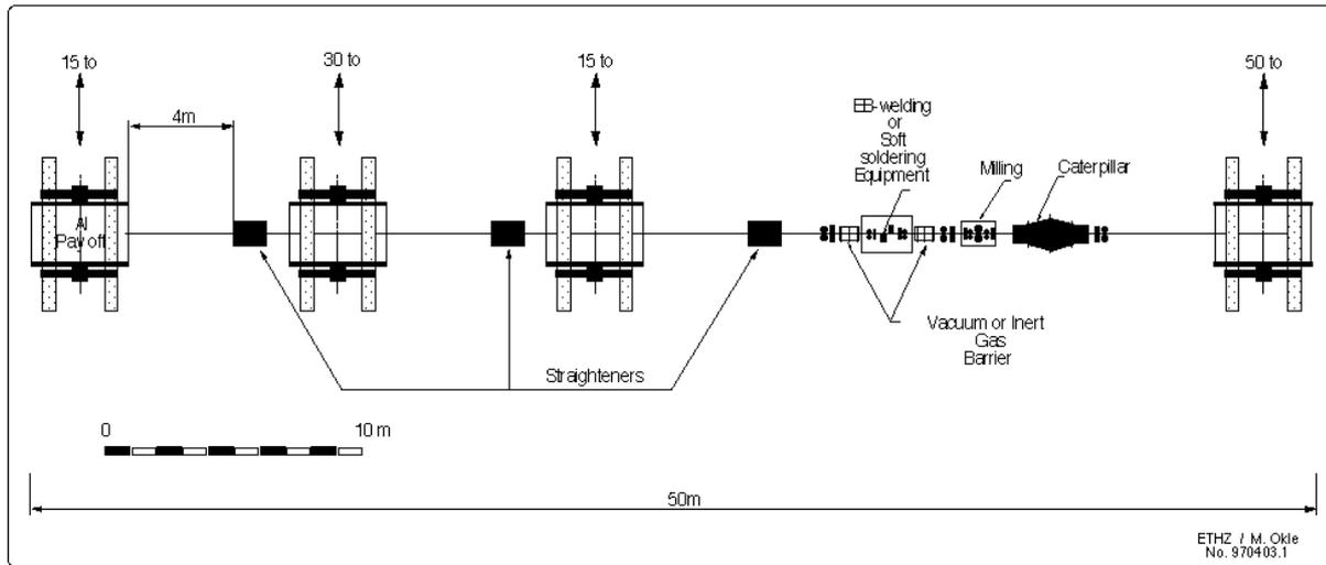
**Fig. 23.1:** Process line for the final CMS conductor manufacturing.
