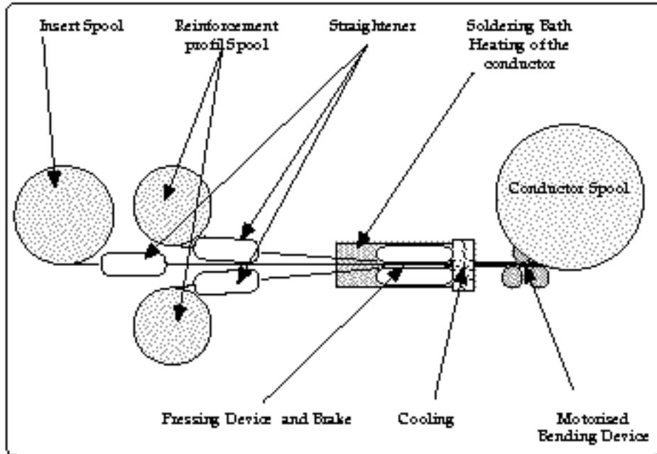
**Fig. 23.9:** Continuous soldering principle.
