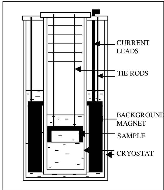
**Fig. 23.6:** Schematic view of the MA.R.I.S.A. test facility.
