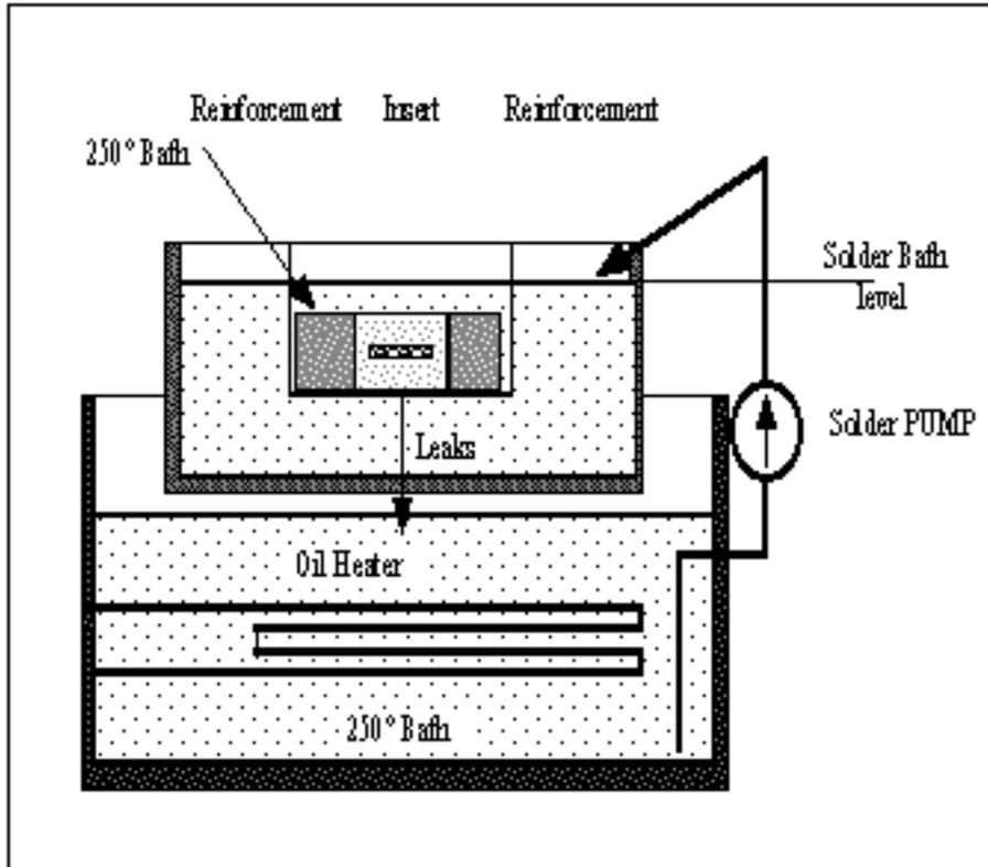
Fig. 23.10: Bath principle component side.
