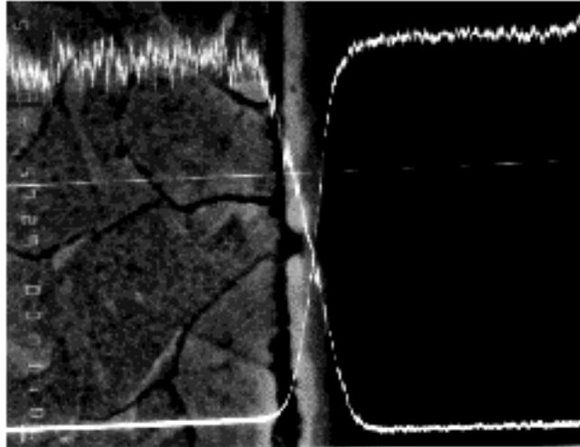
**Fig. 23.3:** Microphotograph of the conductor cross section. Between the etched copper matrix of the superconductor strands and the aluminium surface of the stabiliser, a diffusion layer of 3  $\mu\text{m}$  thickness can be seen.
