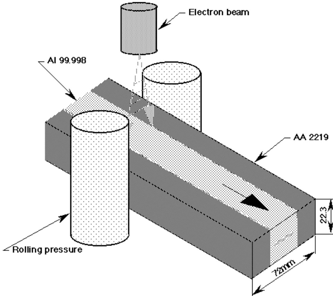
**Fig. 23.8:** Scheme of the Electron Beam Welding System.
