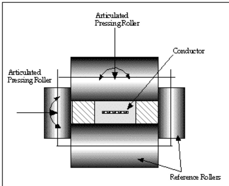
**Fig. 23.12:** Pressing system in the soldering Bath.
