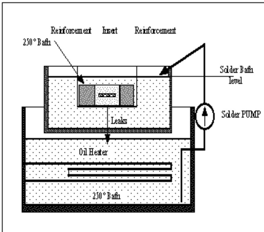
Fig. 23.11: Bath principle assembled conductor side.
