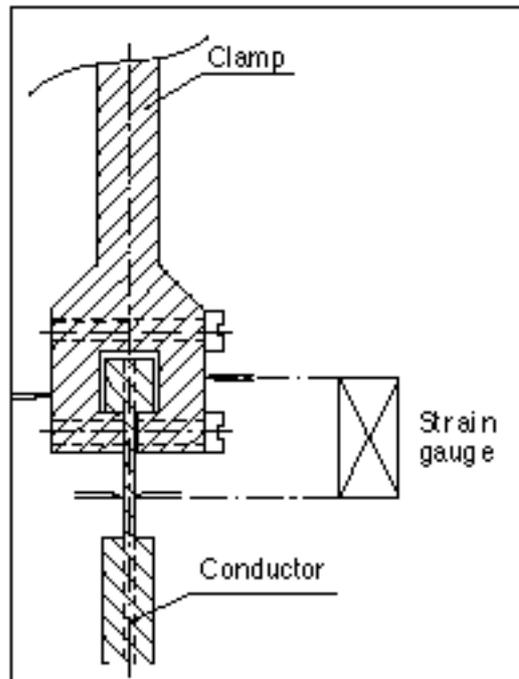
Fig. 23.2: Tooling for mechanical bond measurements.
