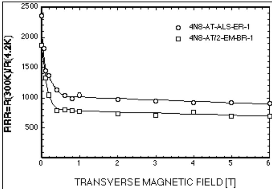
**Fig. 23.5:** The residual resistivity ratio of 4N8 (99.998%) aluminium stabiliser vs. transverse applied magnetic field from the ATLAS conductor delivered by GEC-ALSTHOM (ALS-ER-1) and Europa Metalli (EM-BR-1).
