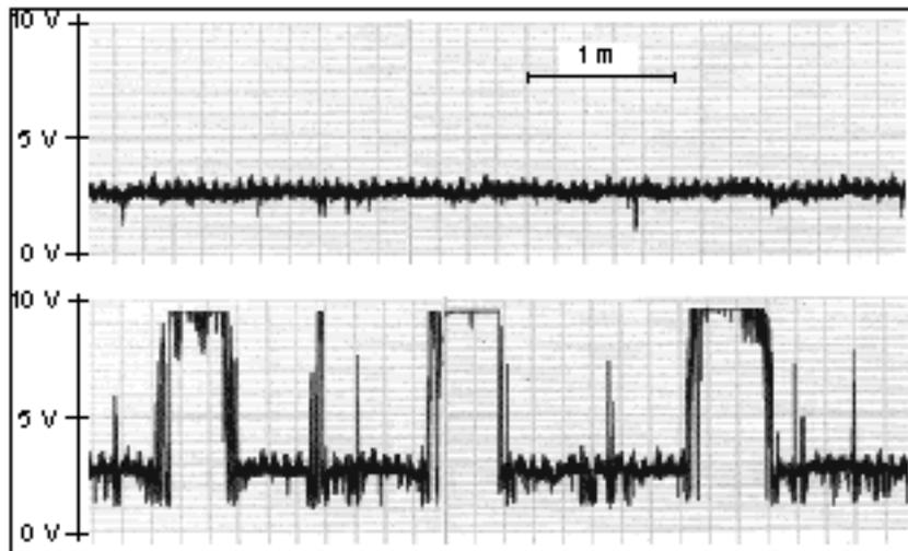
**Fig. 23.7:** Continuous ultrasonic testing of bond-quality of the Fermilab D0 cable.
