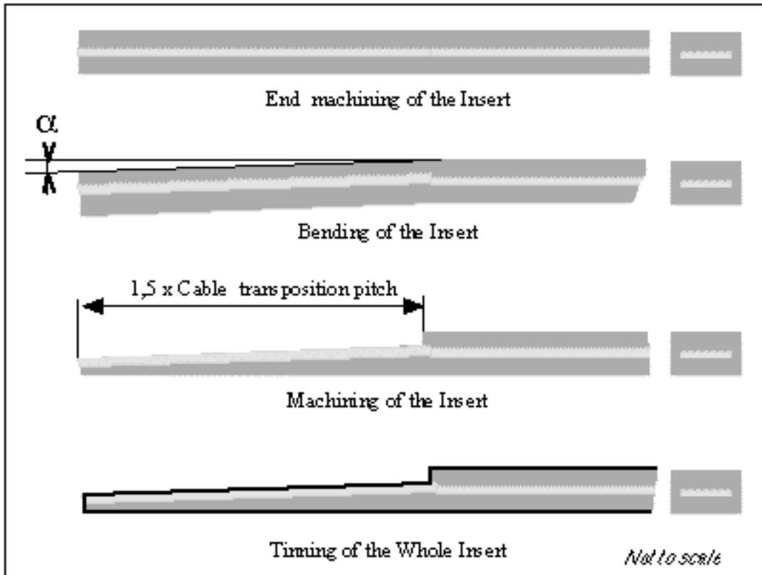
**Fig. 23.13:** Machining and tinning of an insert end to prepare for a joint. An alternative way is to leave 5 mm of pure aluminium over the insert and use EB welding.
