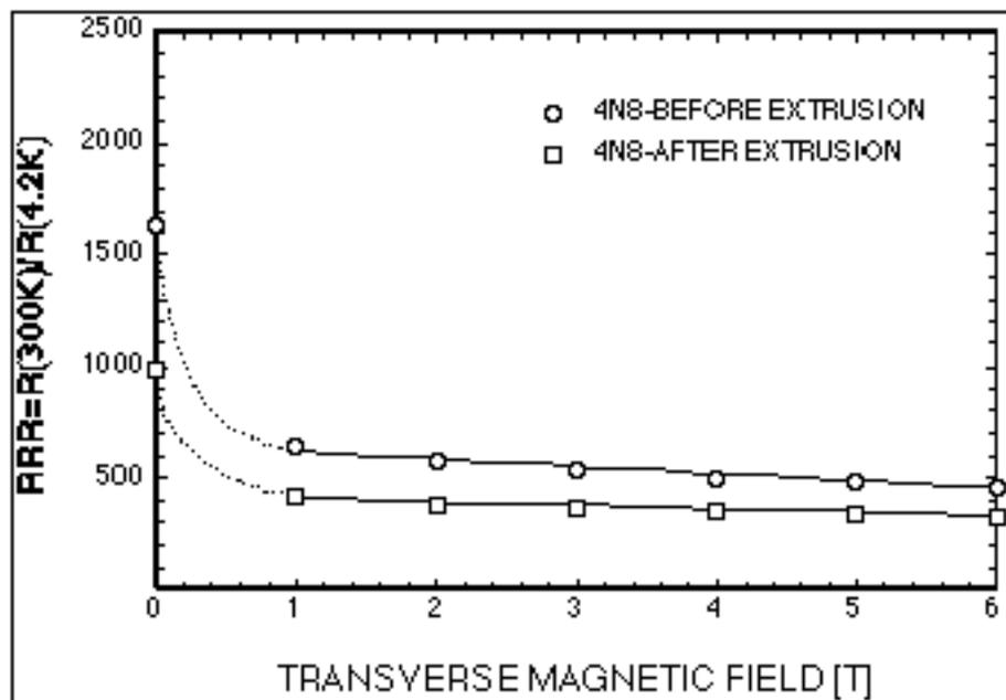
**Fig. 23.4:** The residual resistivity ratio of 4N8 (99.998%) aluminium vs. transverse applied magnetic field before and after extrusion.
