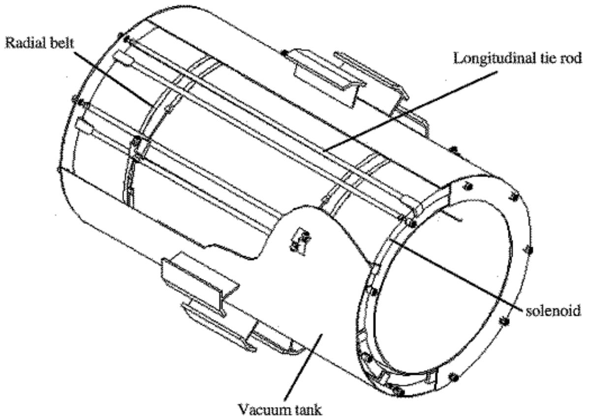
**Fig. 18.1:** General view of the support system.
