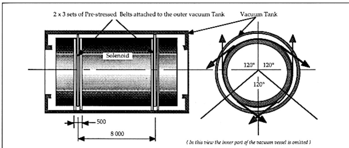
**Fig. 18.4:** Radial positioning system of the solenoid.
