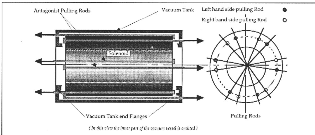
**Fig. 18.3:** Longitudinal positioning system of the solenoid.
