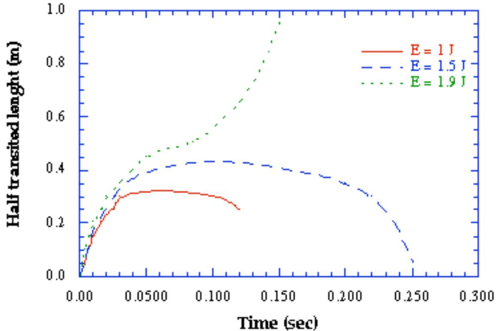
**Fig. 15.7:** Time evolution of the normal zone in the case of finite current diffusion for the ALEPH coil.
