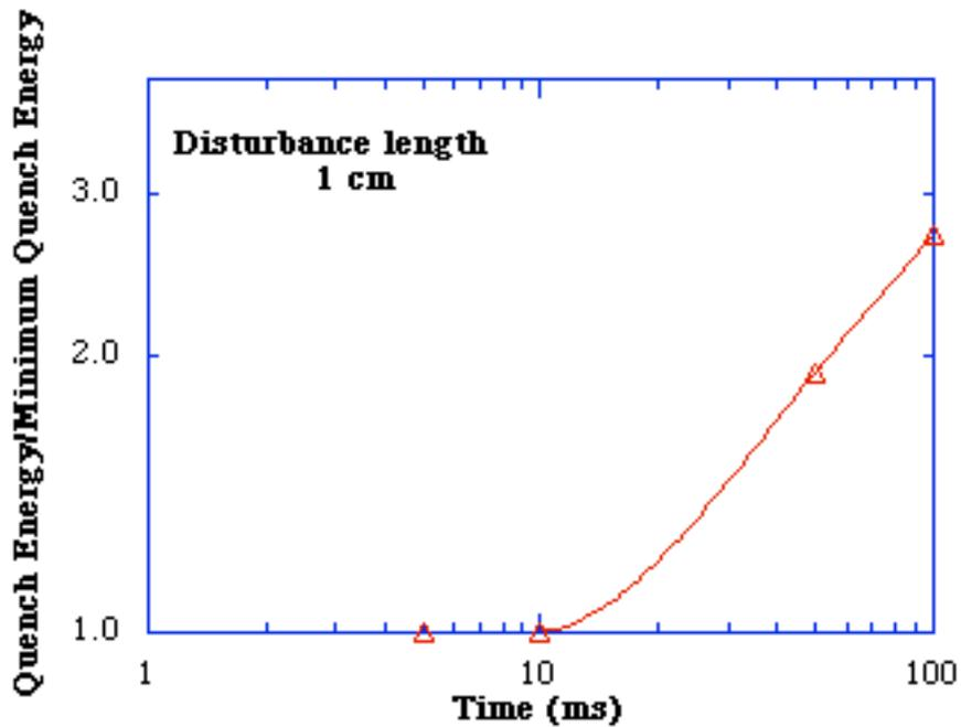
**Fig. 15.9:** Quench Energy vs. the disturbance duration at a fixed value of the disturbance length (1 cm).
