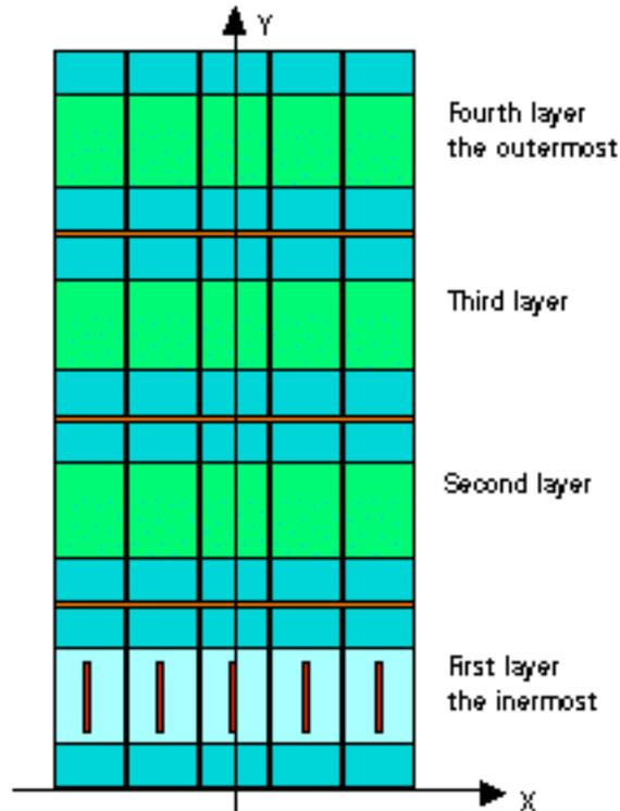
**Fig. 15.4:** Cross section (plane x-y equivalent to the z-r plane) of the CMS winding model.
