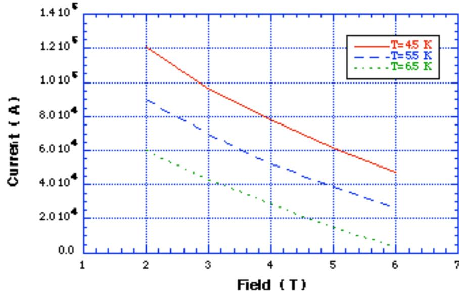
**Fig. 15.1:** Critical current Vs magnetic field at 3 different temperatures, intercepting the peak field load line.
