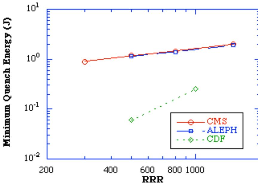
**Fig. 15.12:** MQE vs. RRR for CMS, CDF and ALEPH solenoids in the case of finite current diffusion.
