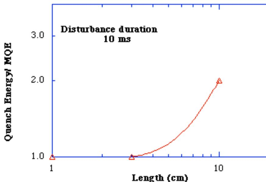
**Fig. 15.10:** Quench Energy Vs the disturbance length at a fixed value of the disturbance duration (10 ms).
