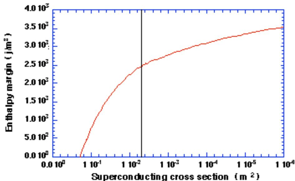
**Fig. 15.2:** Enthalpy margin Vs the superconducting cross section.
