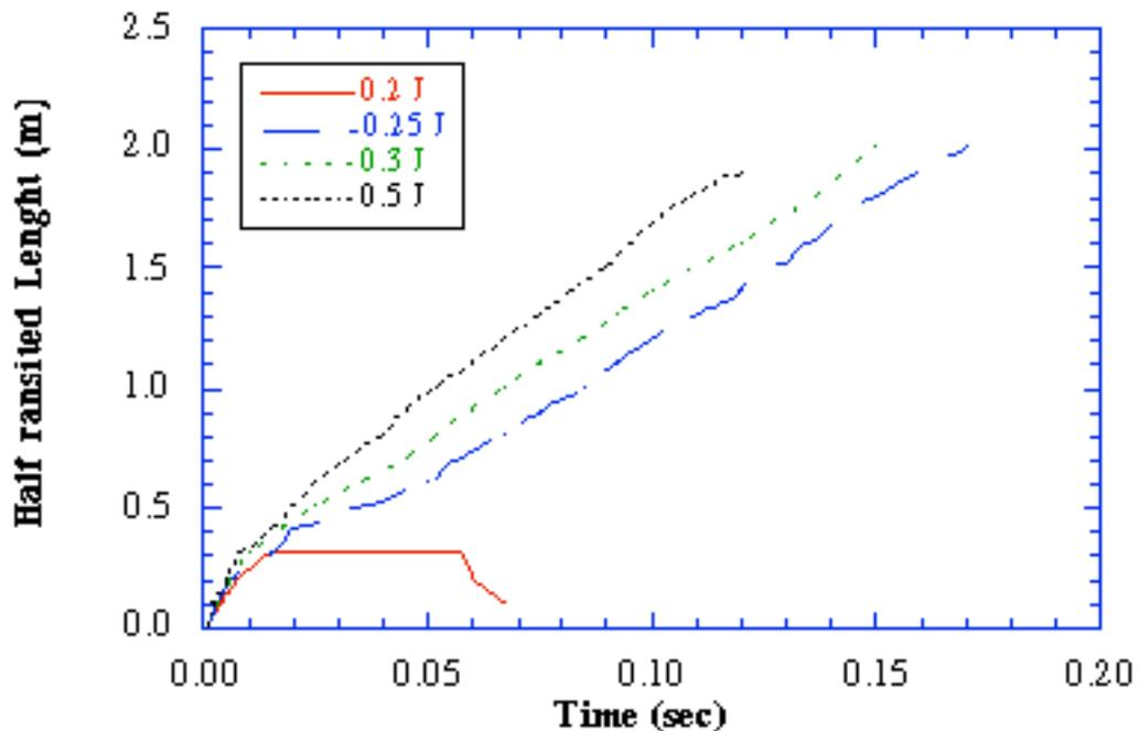
**Fig. 15.8:** Time evolution of the normal zone in the case of finite current diffusion for CDF coil.
