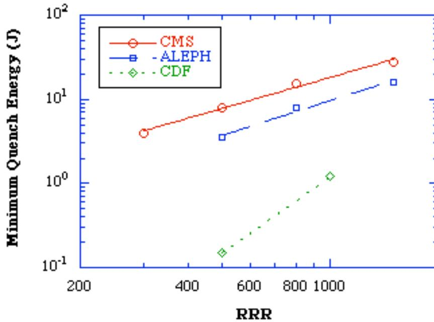
**Fig. 15.11:** MQE vs. RRR for CMS, CDF and ALEPH solenoids in the case of instantaneous current diffusion.
