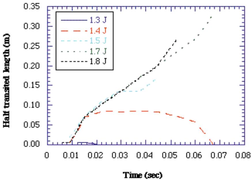
**Fig. 15.6:** Time evolution of the normal zone in the case of finite (and real) current diffusion.
