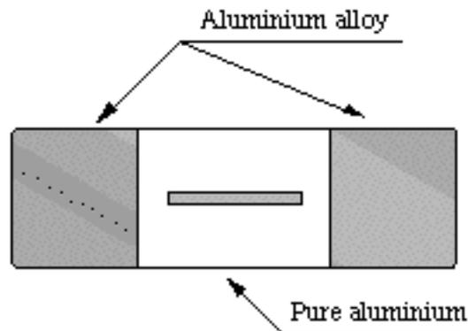
**Fig. 11.1:** Block conductor geometrical arrangement.
