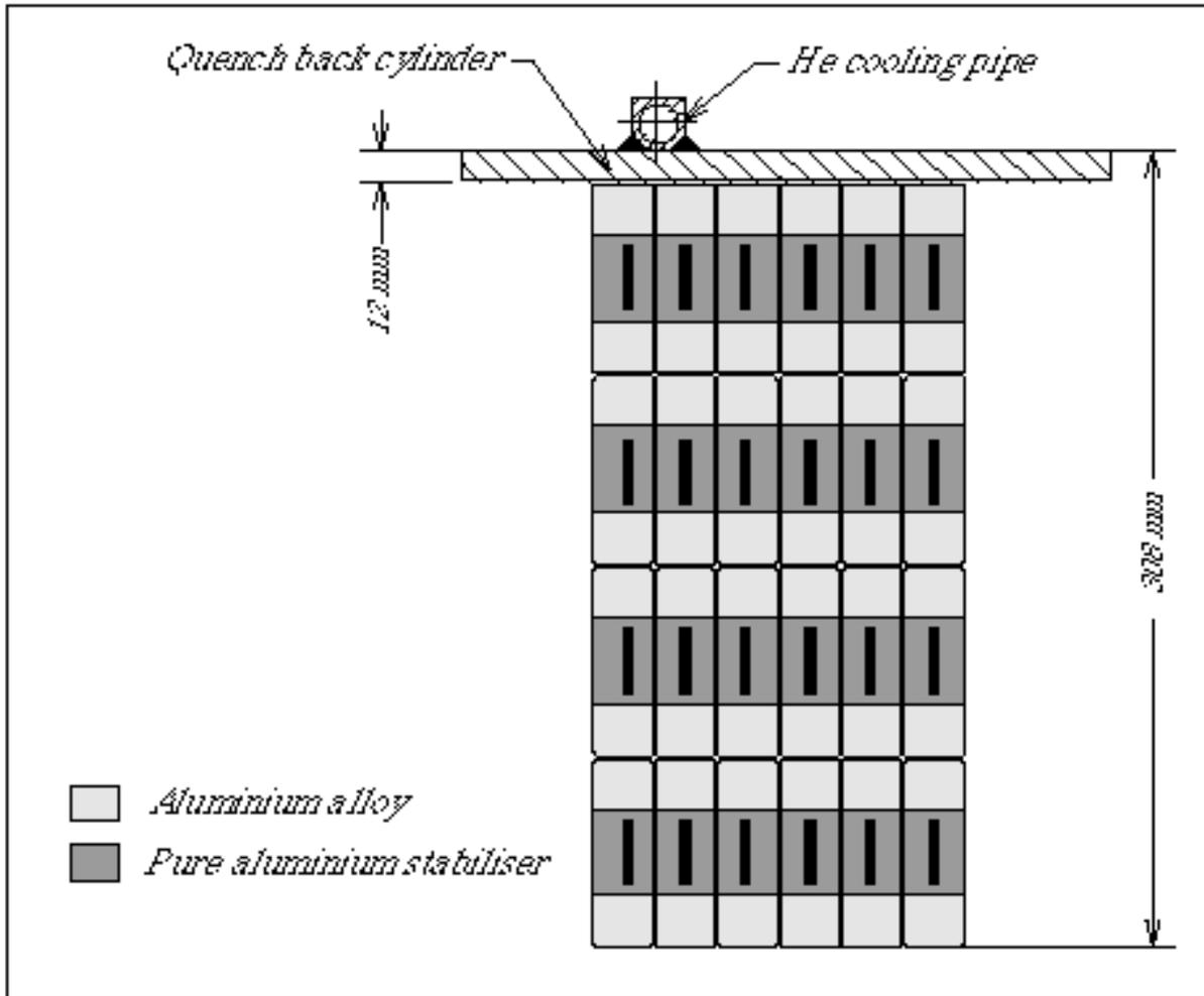
**Fig. 11.2:** View of the winding showing the structure in concentric cylinders.
