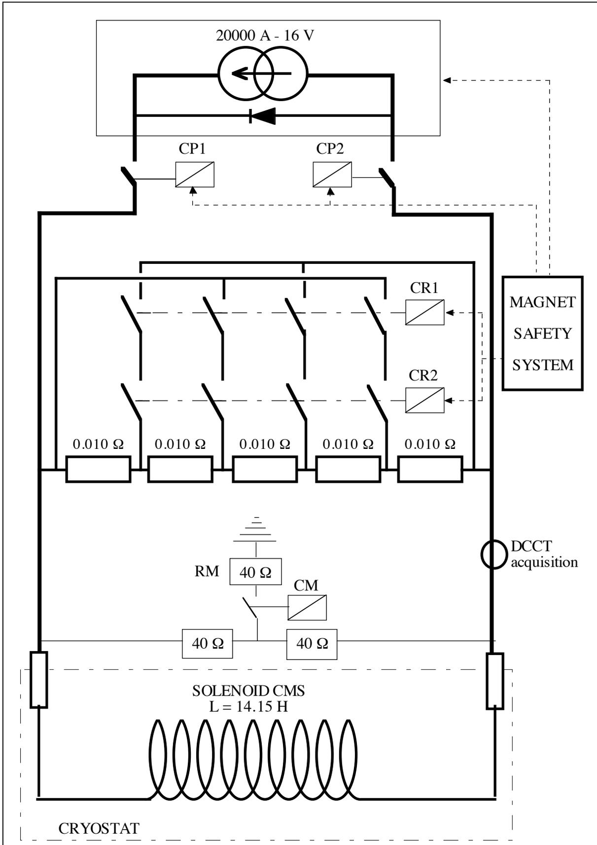
Fig. 20.1: Electrical circuit for the CMS solenoid.
