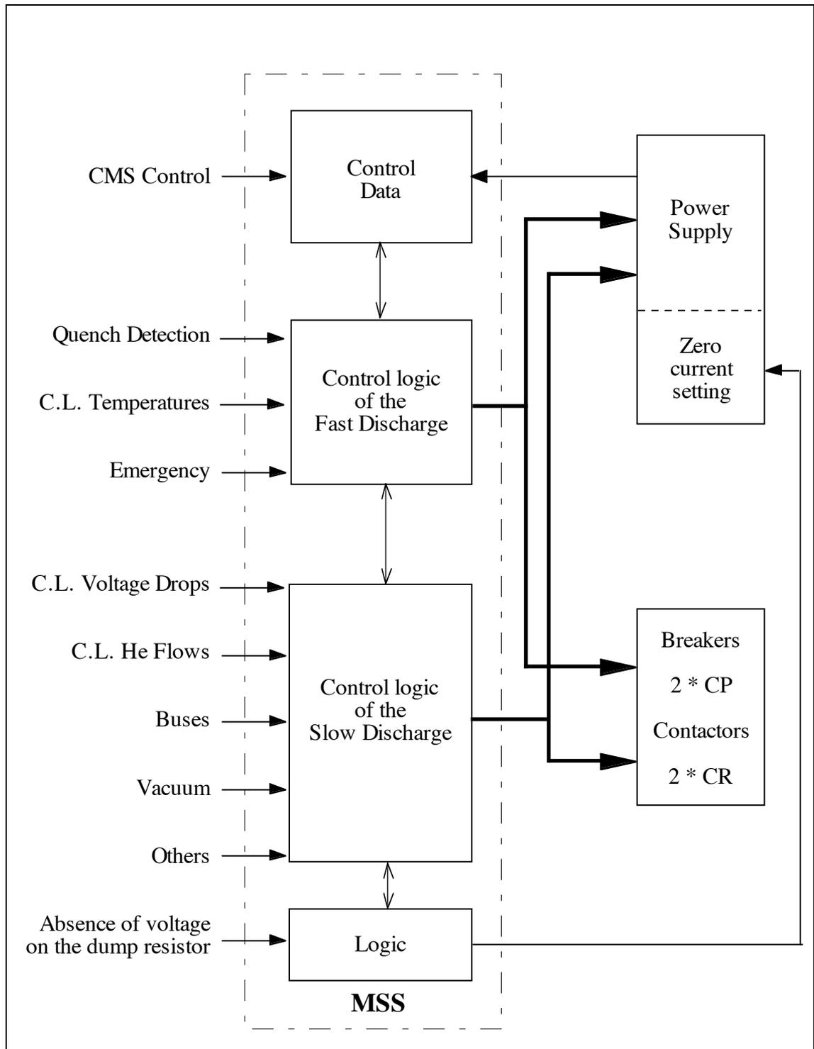
**Fig 20.2:** Diagram of the Safety Interlocks.
