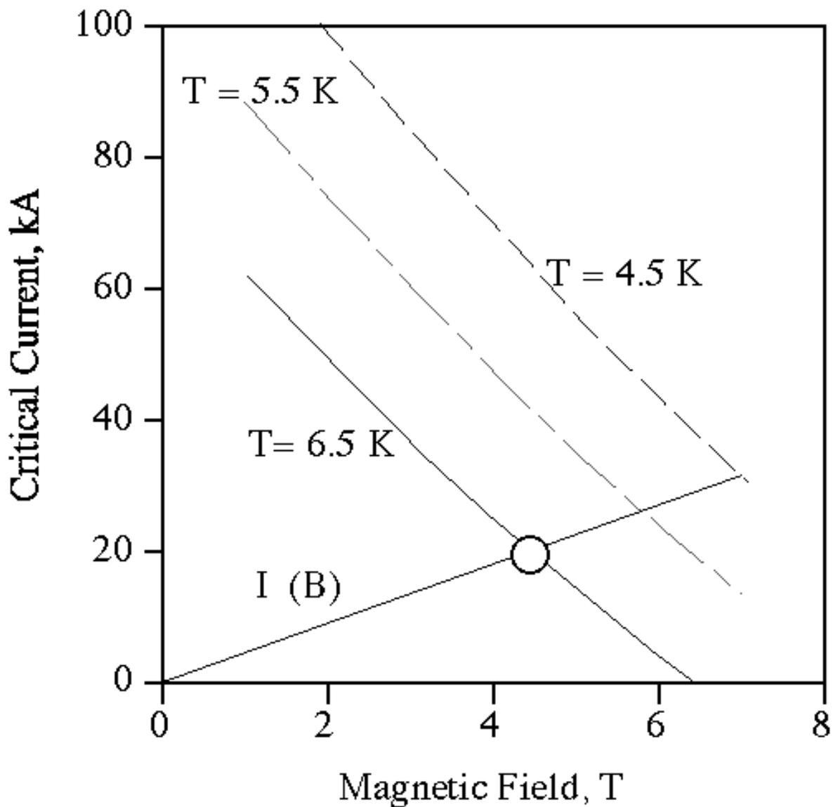
**Fig. 12.3:** CMS conductor current - field diagram.
