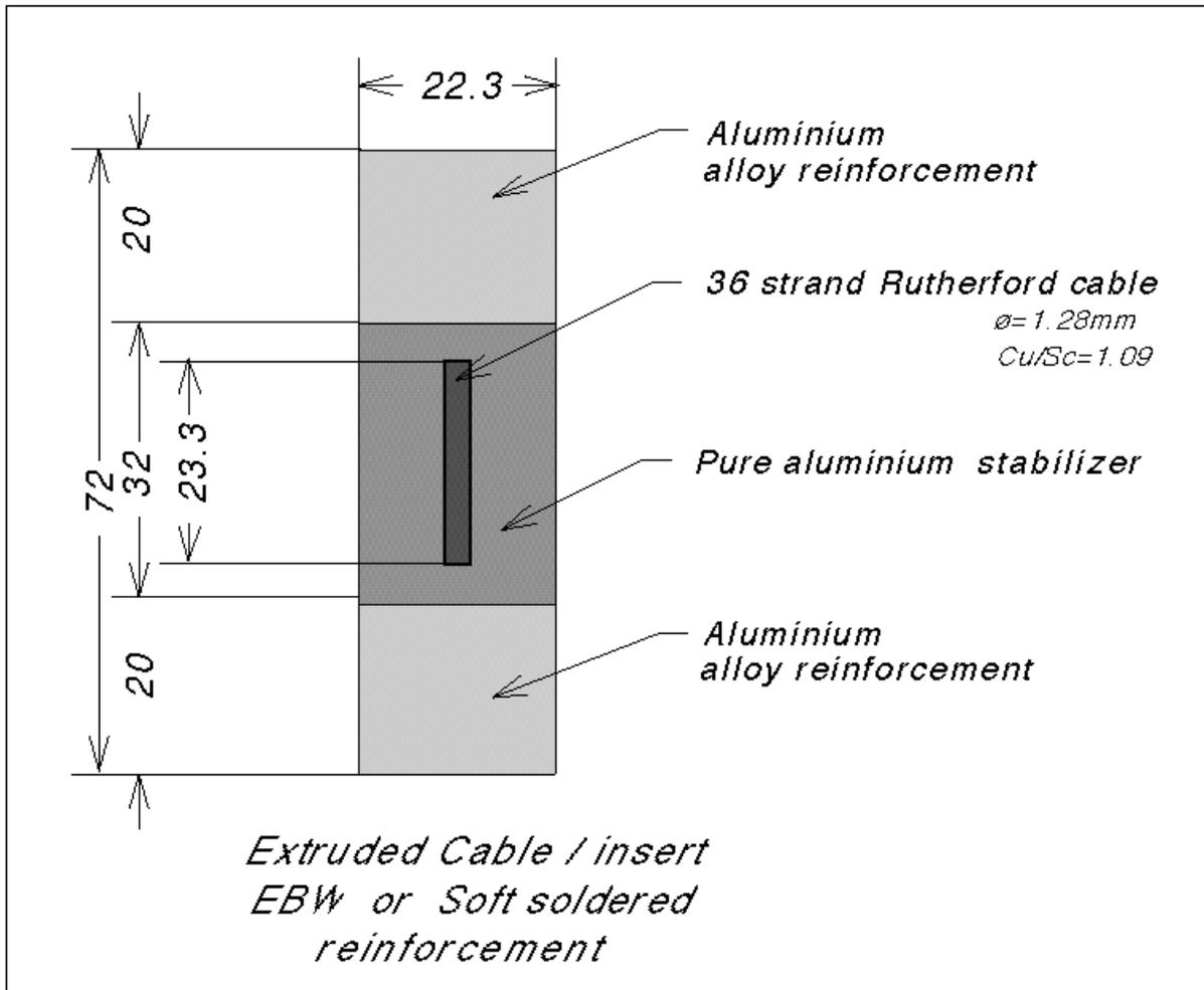
Fig. 12.1: Conductor cross section.
