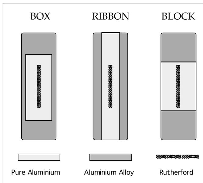
**Fig. 12.2:** Conductor geometrical configurations.
