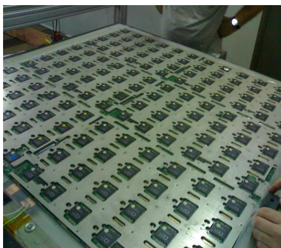
Figure 16: HARDROC integration on slab @ IPNL
