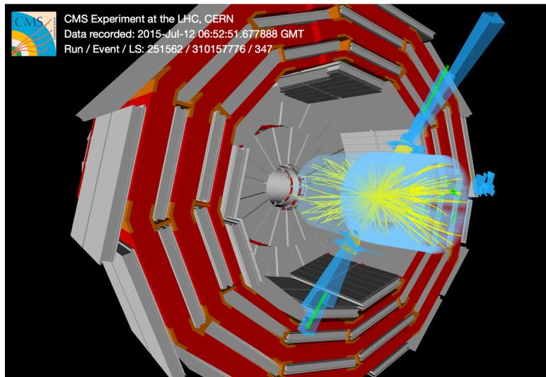
A 13TeV collision recorded by the CMS detector showing two high-energy particle jets with a collective mass of 5 TeV
